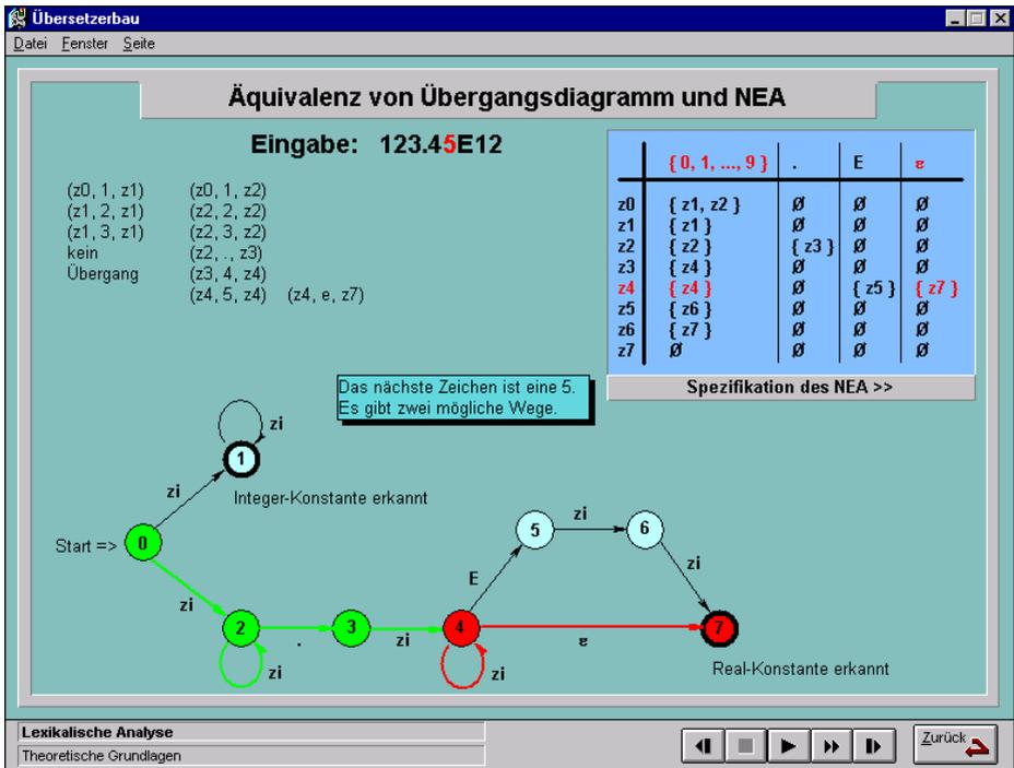
Fig. 1. Equivalence of Transition Diagram and NFA
