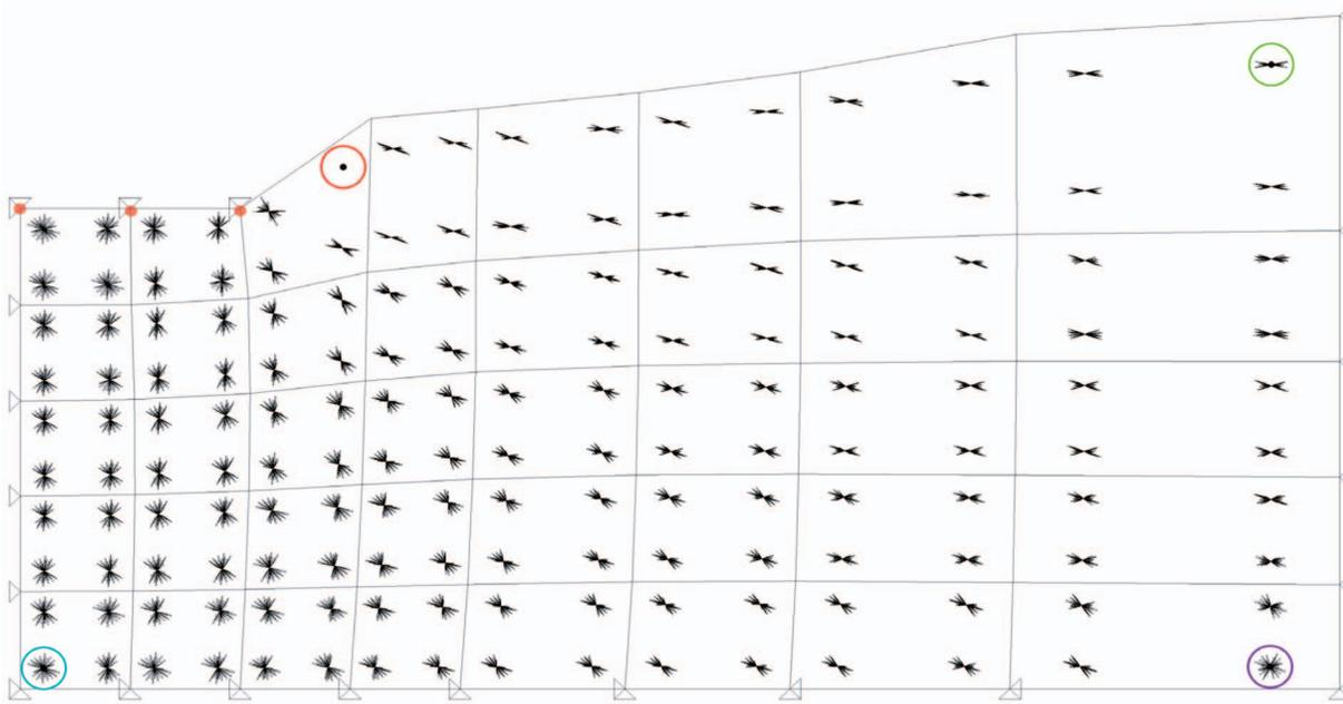
Fig. 12. Macroscale-Level View of the *final* deformed state. 40 finite elements are used to discretize one half of the footing problem. Red dots were manually added to this screen shot to point at the three nodes displaced by the footing. Boundary conditions are applied by displacements of the restricting bearings. Glyphs are visible and give a good overview of the underlying microstructure. All rves of the user selected and marked Gauss points are depicted in Fig. 13.
