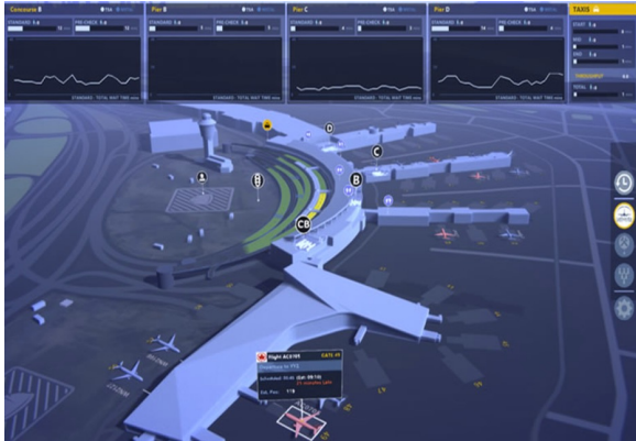
SITA's digital twin for airport operations control
