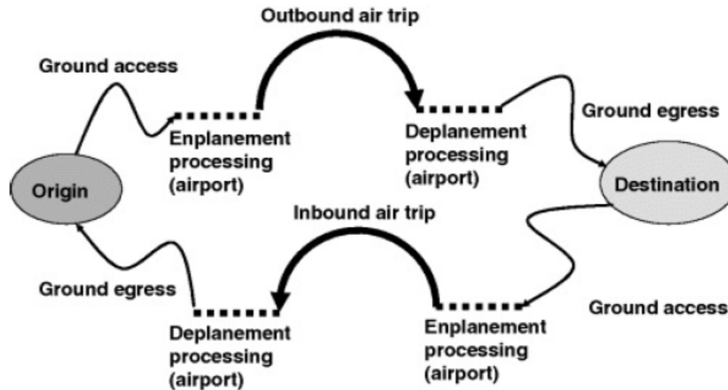
**Figure 3.1** Representation of a typical air passenger trip
