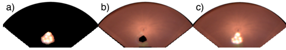
Figure 8: a) A light source SLF extracted and separated from an ILF. b) The residual background ILF with missing data. c) The sum of the influence of both the SLF and the ILF.
